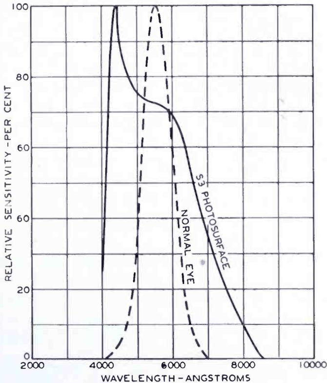
Fig. 2—Spectral distribution of the S3 surface. Spectral sensitivity of the human eye.
