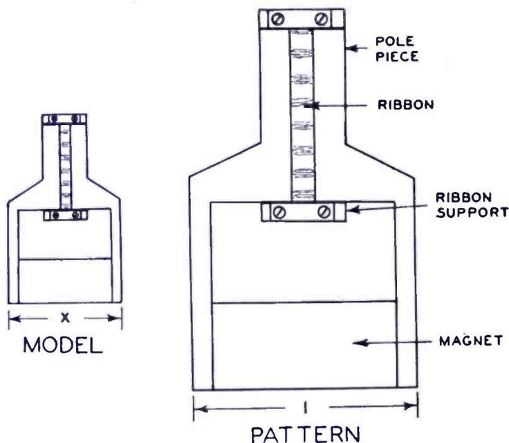
Fig. 1—Two similar velocity microphones with linear dimensions in the ratio of  $x:1$  termed the model and pattern, respectively.
