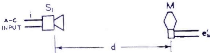
Fig. 3—Arrangement for obtaining the open-circuit voltage  $e'_M$  of the microphone when driven by a pressure  $p$  produced by the microphone-loudspeaker actuated by a current  $i$ .
