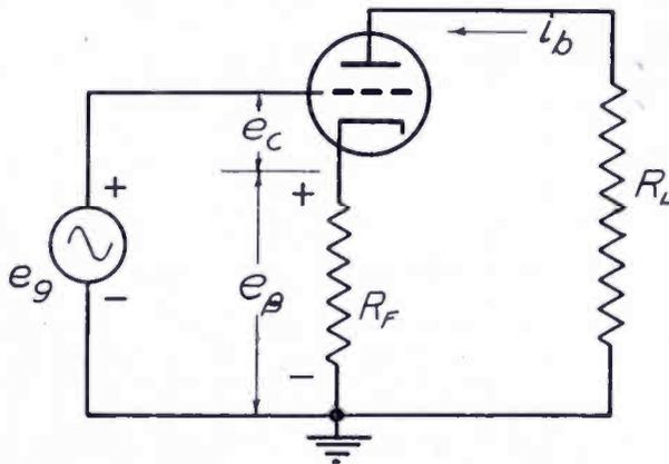
Fig. 6—Negative current feedback
