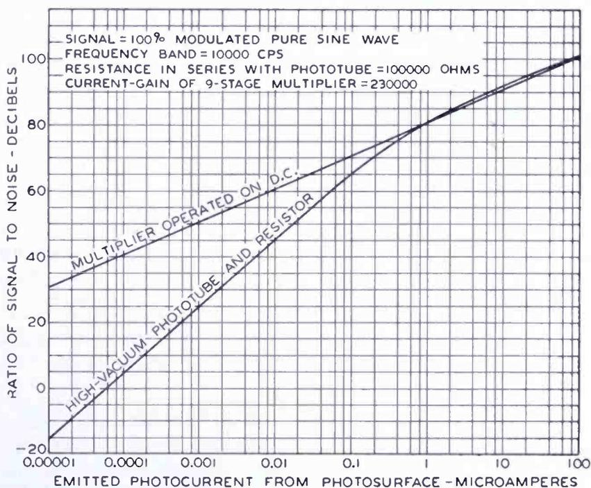
Fig. 8—Signal-to-noise ratio of a multiplier phototube.
