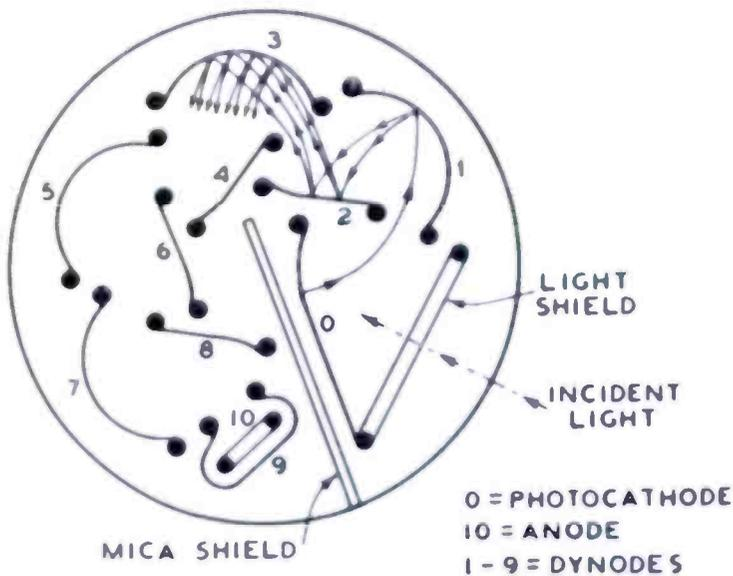
Fig. 7—Internal structure of the 931.
