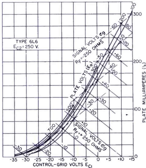
Fig. 7—Transfer characteristics of Type 6L6 with construction for obtaining current feedback characteristics
